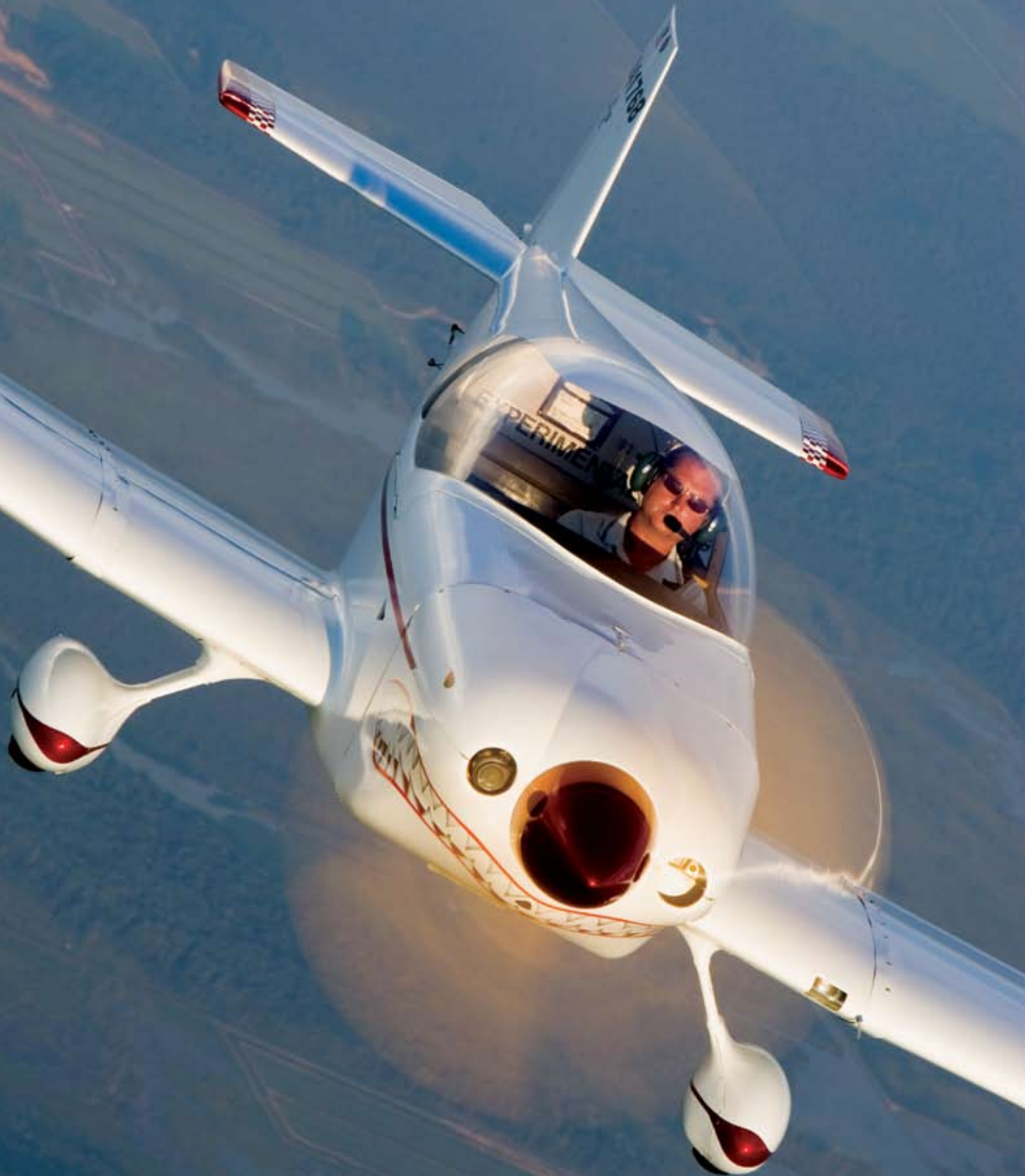
Bill Clapp's red-on-white KR-2S hides a 100-hp Corvair engine under its shark-tooth cowl.
